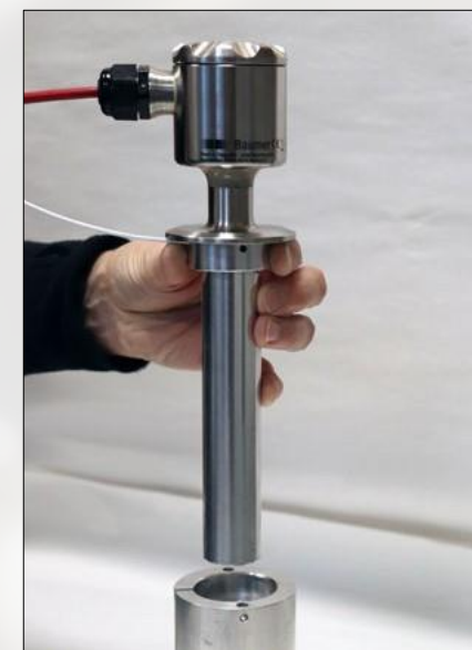
Assembled RTC-156 insert and RTC-158 adapter.
